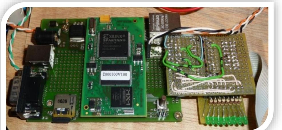
ARM 200Mhz, FPGA (SPARTAN3E), RJ45, I2C ADC/DAC, GPIO, ...
