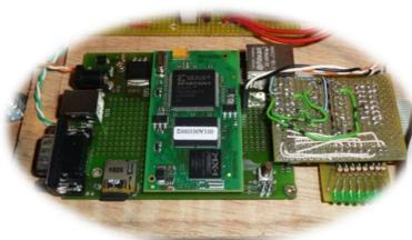
ARM 200Mhz, FPGA (SPARTAN3E), RJ45, I2C, ADC/DAC, GPIO, ...
